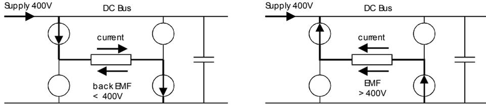
(a) Electrical power to motor      (b) Electrical power from motor (regeneration)
