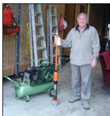
Figure 7: Air Compressor and Backfill Tamper
