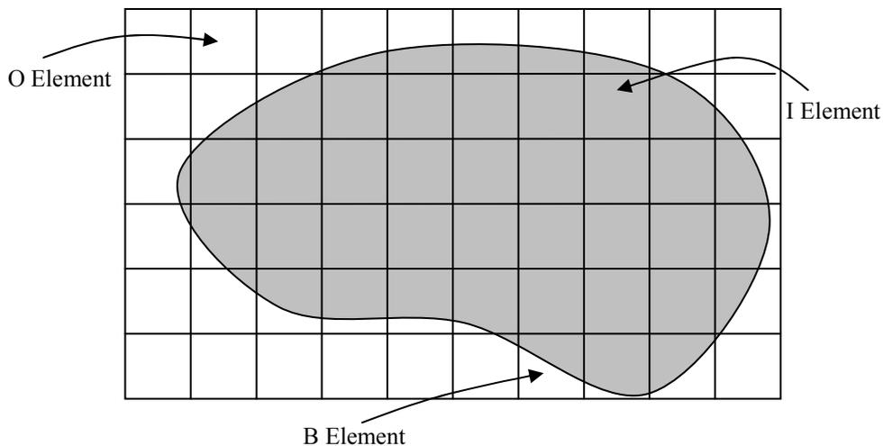
Figure 1: Fixed grid domain with superimposed topology in grey, showing inside (I), outside (O) and Boundary (B) elements
