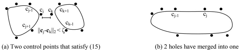
Figure 10: An example of merging two holes
