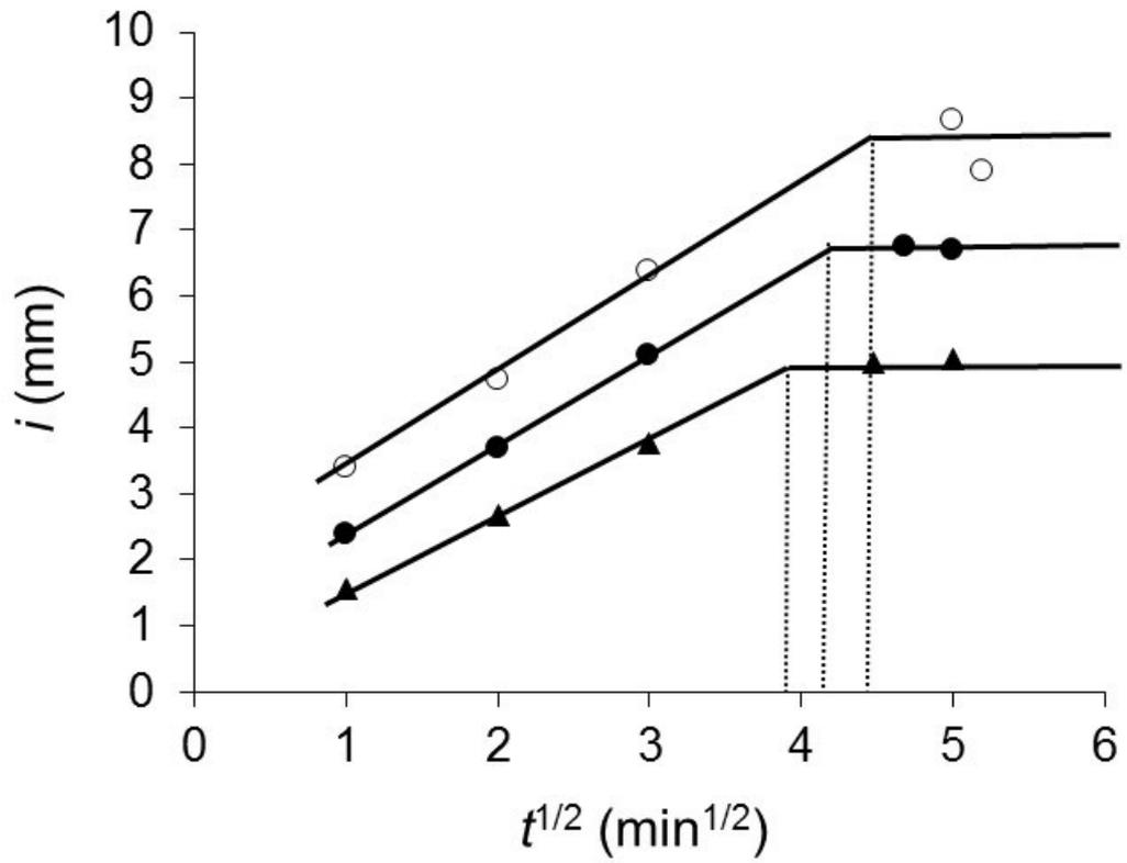
Figure 6. Water absorbed by a brick substrate from a range of wet mixes of varying water content: cumulative absorbed volume per unit area  $i$  versus  $t^{1/2}$  for NHL 2 mortars of binder: sand ratio 1:2 with water: binder ratios ▲, 0.78:1; ●, 0.89:1; and ◻, 1:1.
