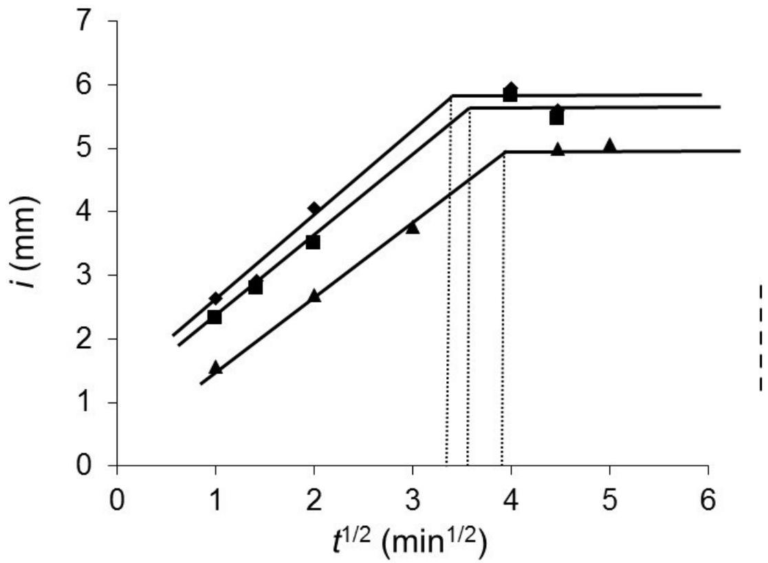
Figure 5. Water absorbed by a brick substrate from a range of wet mixes of varying hydraulicity: cumulative absorbed volume per unit area  $i$  versus  $t^{1/2}$  for ▲, NHL 2; ■, NHL 5; and ◆, OPC mortars all of mix composition water: binder: sand 0.78:1:2 by volume.
