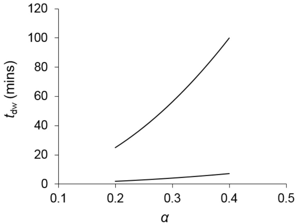
Figure 2. Theoretical plots of Eq. (3) for a high transfer sorptivity ( $A = 3 \text{ mm/min}^{1/2}$ , lower line) and a low transfer sorptivity ( $A = 0.8 \text{ mm/min}^{1/2}$ , upper line).  $t_{dw}$  calculated using  $L = 20 \text{ mm}$  with  $\alpha$  in the range 0.2 to 0.4 in each case.
