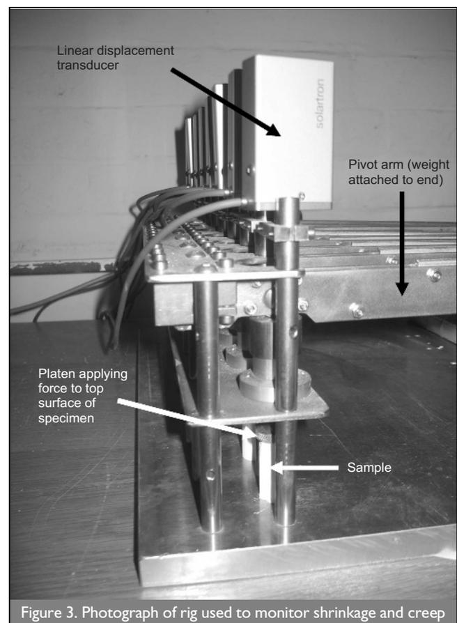
Figure 3. Photograph of rig used to monitor shrinkage and creep
