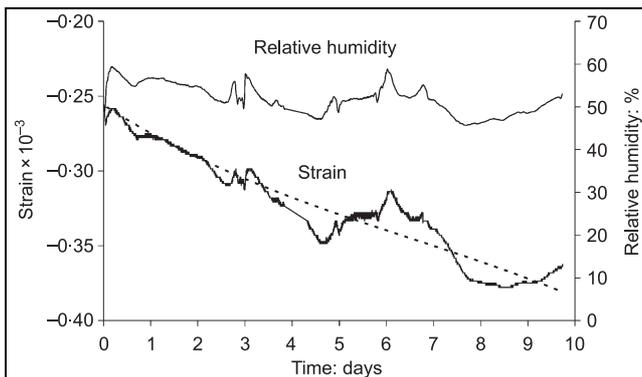
Figure 5. Deformation and relative humidity of a 90-day-old sample of NHL3.5 over a period of 10 days
