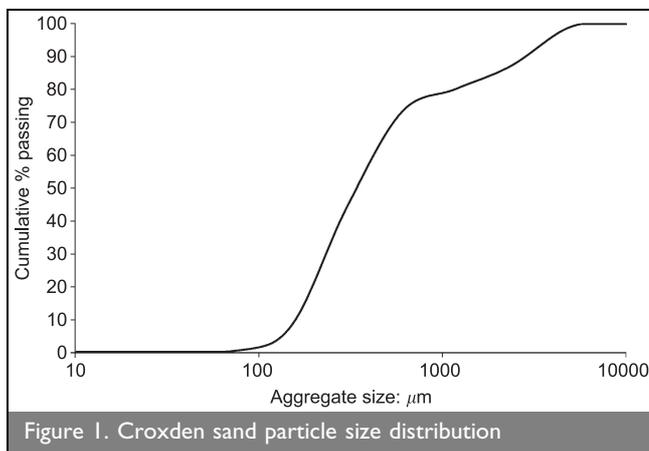
Figure 1. Croxden sand particle size distribution
