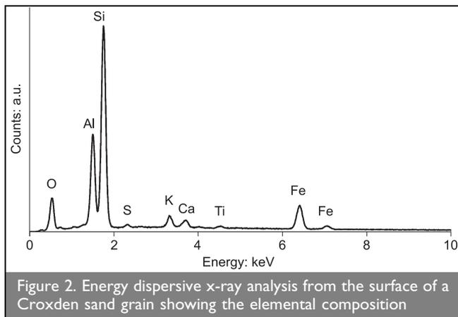
Figure 2. Energy dispersive x-ray analysis from the surface of a Croxden sand grain showing the elemental composition
