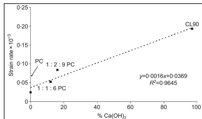
Figure 8. Relationship between strain rate and proportion of calcium hydroxide content by weight
