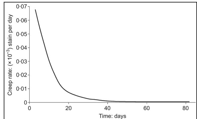
Figure 7. Creep rate observed in 1 : 2 NHL3.5 specimen
