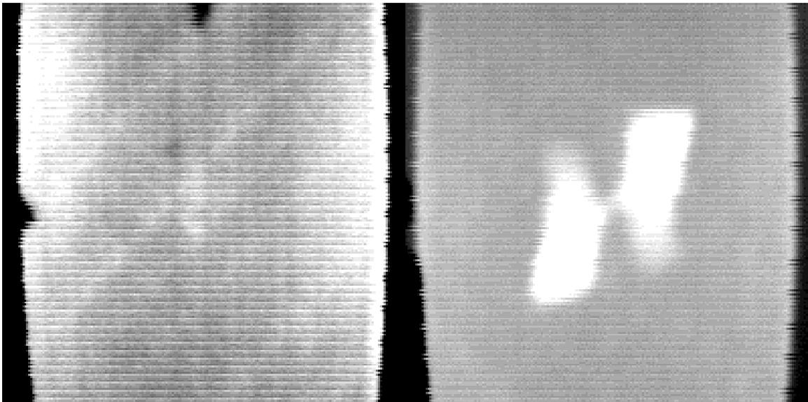
Figure 3 Front, a, and back, b, TT images of an 8 blanket, Painted, High energy impacted laminate
