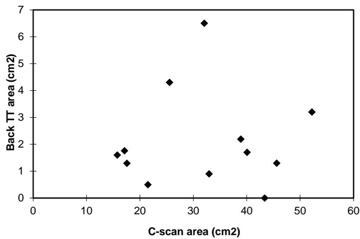
Figure 11 Plot of back TT area vs. UCS area of 4 blanket specimens, a, 8 blanket specimens, b, & 16 blanket specimens, c
