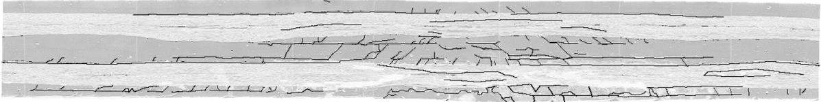
Figure 12 Photo micrograph showing crack network in a 4 blanket laminate
