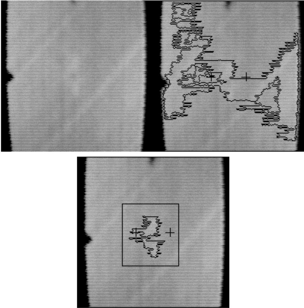
Figure 8 TT images showing defect, a, calculated defect area, b, and calculated defect area using ROI box, c
