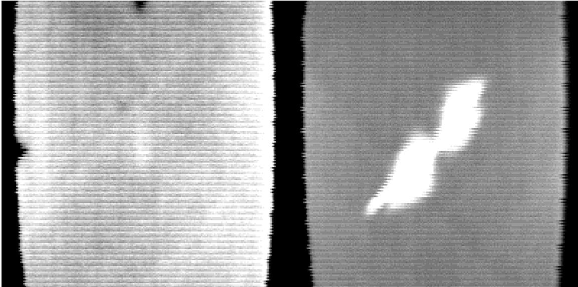
Figure 2 Front, a, and back, b, TT images of a 4 blanket, Painted, High energy impacted laminate
