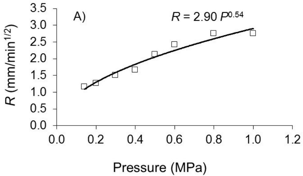
Figure 2. Variation in desorptivity with applied pressure. A: □, CL 90 mortar of composition 0.78:1:2 water: binder: sand; B: ●, NHL 2 mortar of composition 1:1:2 water: lime: sand (upper line) and 0.78:1:2 water: lime: sand (lower line).
