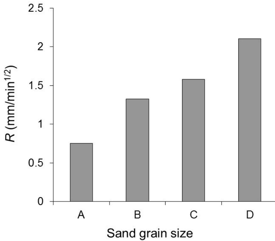
Figure 8. Desorptivity of NHL2 mortars of constant 0.78:1:2 water: binder: sand mix proportions prepared with different grain sizes of sand. A, 75 - 300  $\mu\text{m}$ ; B, 150 - 300 $\mu\text{m}$ . C, 300 - 600  $\mu\text{m}$ ; D, 75 - 600  $\mu\text{m}$ . The applied pressure was 0.05 MPa in each case.
