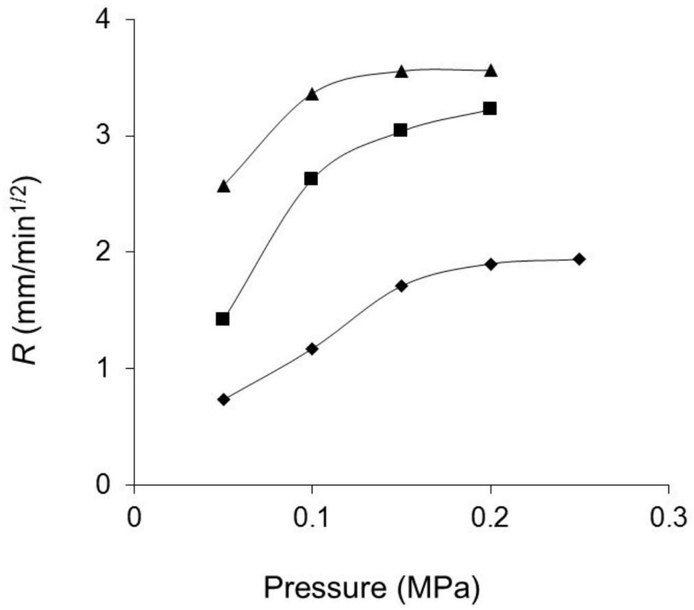
Figure 3. Variation in desorptivity with applied pressure for a range of freshly mixed mortar types all of composition 0.78:1:2 water: binder: sieved sand. ▲, OPC; ■, NHL5; ◆, NHL3.5.
