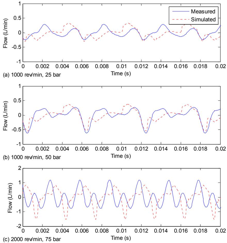
**Figure 4 – Measured and simulated outlet flow ripple**
