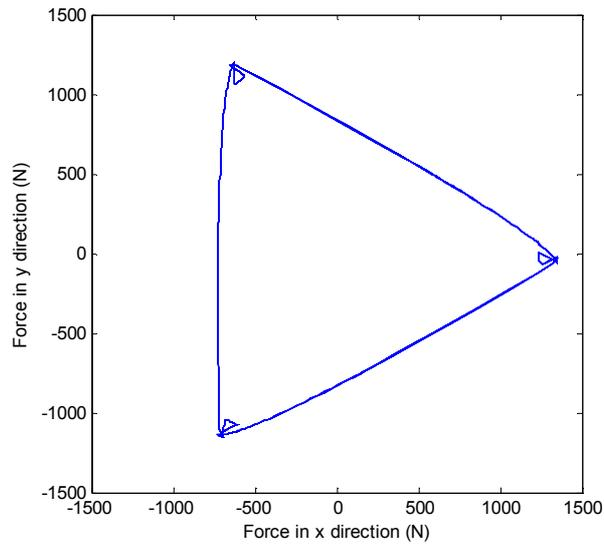
**Figure 13– Resulting lateral forces on rotor, three-port design.**
