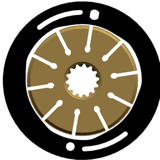
**Figure 9 – Three-port cam ring internal profile.**
