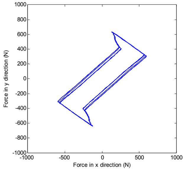
**Figure 12 – Resulting lateral forces on rotor, nine-vane design.**
