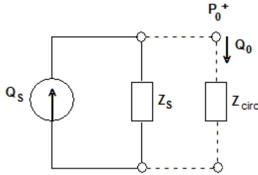
**Figure 2 – Norton model of a pump.**
