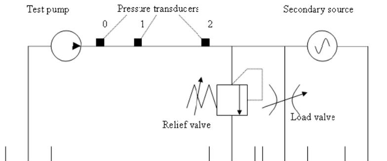
**Figure 3 – Hydraulic Circuit for secondary source method [3].**
