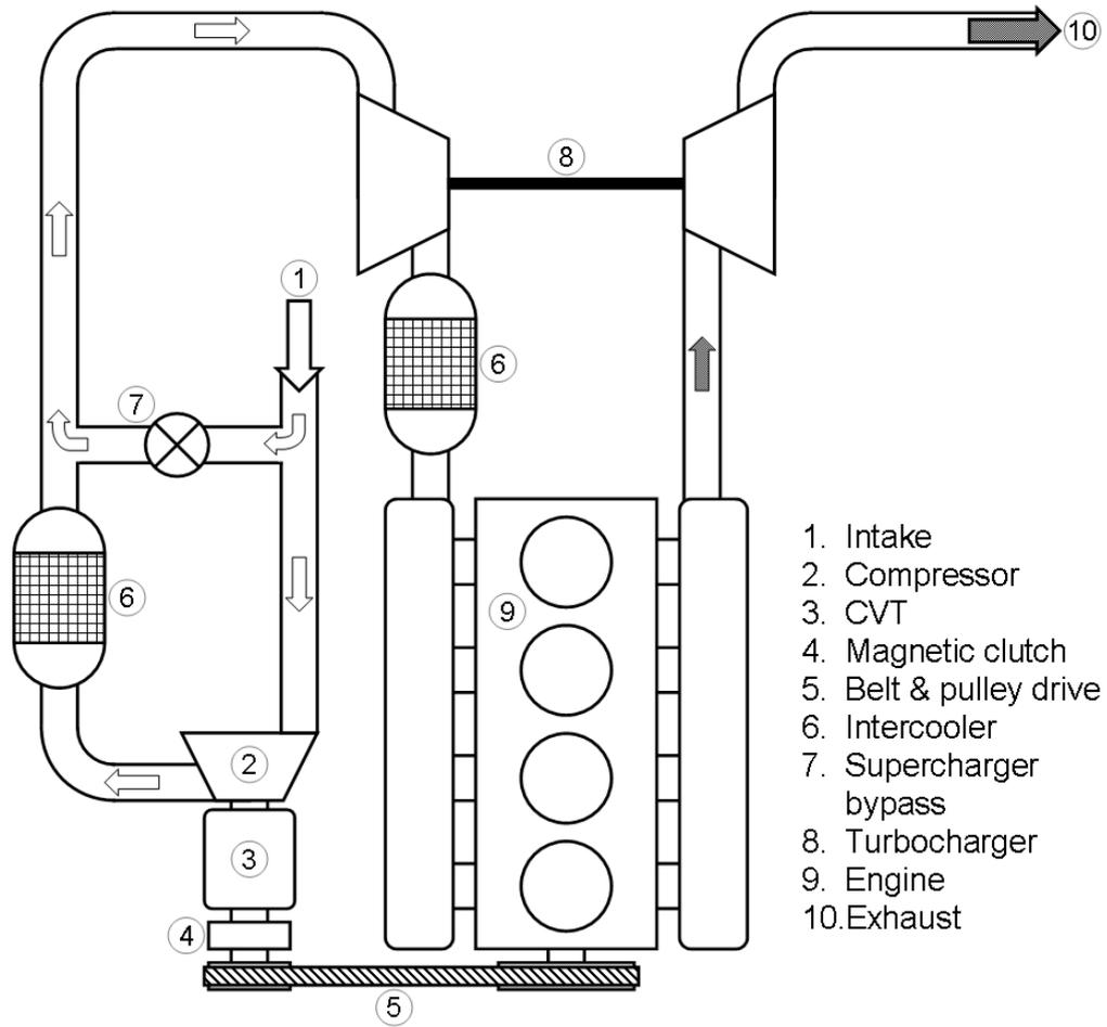
Figure 1 Schematic diagram of the proposed twincharged engine
