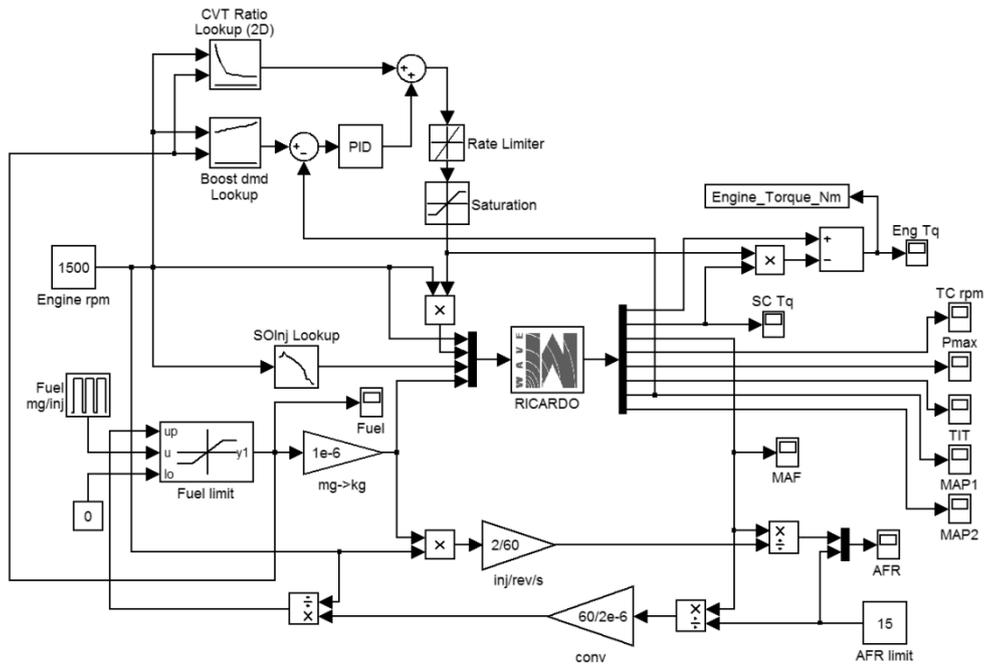
Figure 9 Simulink block diagram – twincharged engine
