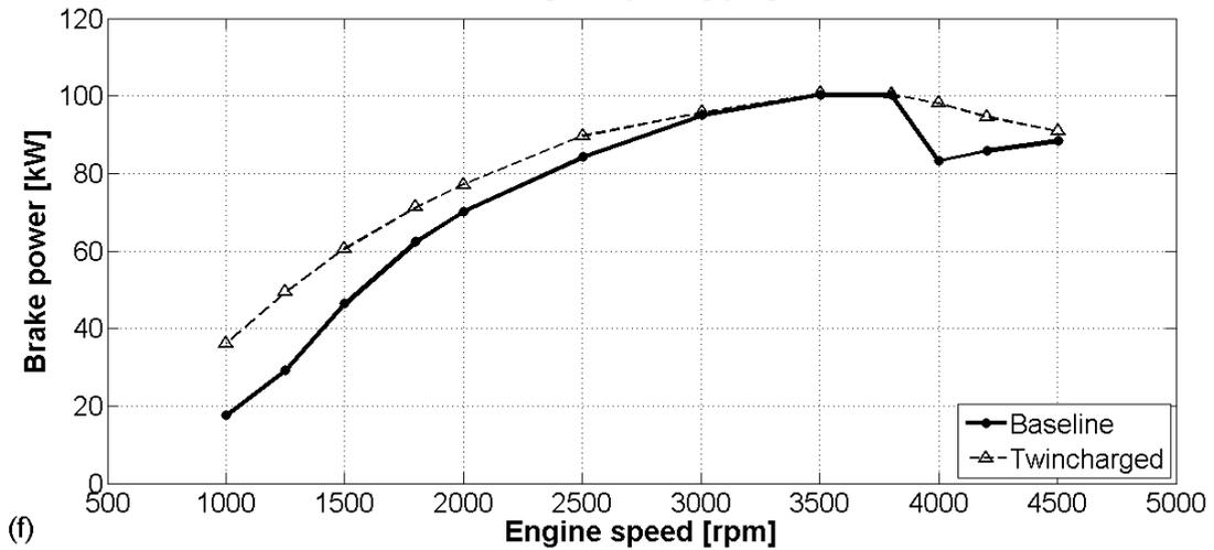
Figure 2 Steady state results – a) torque; b) baseline VGT rack position; c) air and fuel mass flow; d) AFR; e) fuel injection timing; f) power
