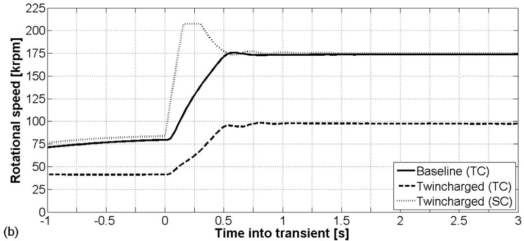
Figure 11 Transient turbocharger and supercharger speeds – a) 1250 rpm; b) 2000 rpm
