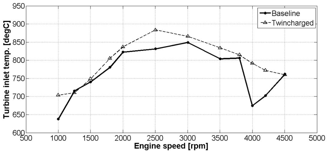
Figure 5 Steady state results – turbine inlet temperature
