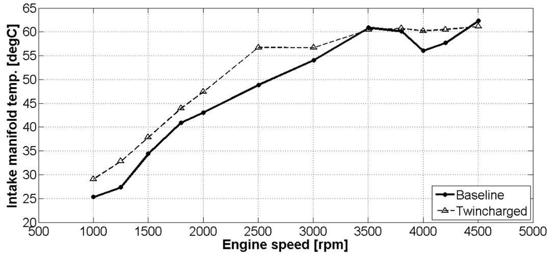
Figure 4 Steady state results – intake manifold temperature
