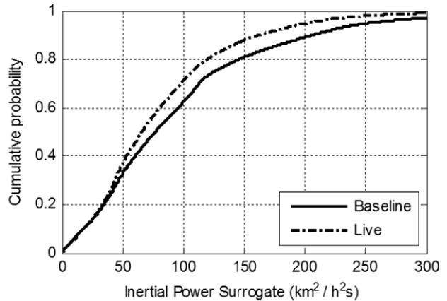
Fig. 7. Cumulative Distribution Functions for positive IPS before and after the device was activated. In the region where  $IPS > 50 \text{ km}^2/\text{h}^2\text{s}$  there is a shift towards lower IPS when the device is active.
