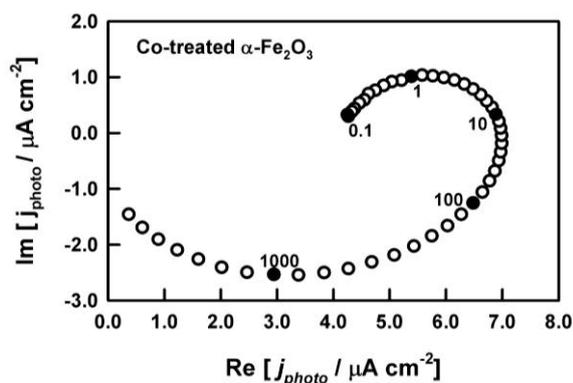
Figure 11. Experimental IMPS response measured for a thin film  $\alpha\text{-Fe}_2\text{O}_3$  electrode in the photocurrent onset region. The electrode was treated with a drop of 10mM cobalt nitrate solution. Electrolyte 1.0 M NaOH. Electrode potential -0.3 V vs. Ag|AgCl. Illumination 455 nm, dc photon flux  $1.1 \times 10^{17} \text{ cm}^{-2} \text{ s}^{-1}$ .
