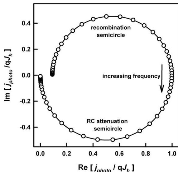
Figure 10. Complete IMPS response including the effects of RC attenuation at high frequencies. Provided that the RC time constant is much shorter than  $(k_{ir} + k_{rec})^{-1}$ , the upper semicircle can be used to derive the two rate constants.
