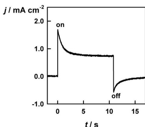
Figure 7. Transient photocurrent response of thin film  $\alpha$ - $\text{Fe}_2\text{O}_3$  electrode at 0 V vs. Ag|AgCl showing the decay and overshoot characteristic of surface electron-hole recombination. Electrolyte 1.0 M NaOH.
