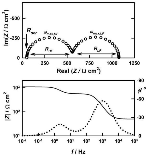
Figure 12. PEIS response predicted for  $k_{tr} = k_{rec} = 10^2 \text{ s}^{-1}$ ,  $J_h = 10^{15} \text{ cm}^{-2} \text{ s}^{-1}$ ,  $C_{sc} = 1 \text{ } \mu\text{F cm}^{-2}$ ,  $C_H = 100 \text{ } \mu\text{F cm}^{-2}$ . The upper complex plane plot shows the two semicircles, and the lower Bode plot shows the separation of the low and high frequency  $RC$  time constants (continuous line: magnitude; broken line: phase).
