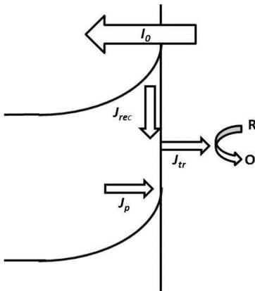
Figure 3. Balance of steady state photon ( $I_0$ ), hole ( $J_p$ ) and electron ( $J_{rec}$ ) fluxes into the semiconductor/electrolyte interface.  $J_{tr}$  is the flux of holes taking part in interfacial electron transfer to oxidize solution species.
