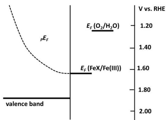
Figure 6.  $\alpha\text{-Fe}_2\text{O}_3$ /electrolyte interface energetics showing possible pinning of hole QFL by a surface iron redox couple. The Fe(X) species here is formed by capture of holes at surface sites. The valence band position is obtained from the flat band potential of hematite and the Fe(X)/Fe(II) redox potential is obtained from the quasi-reversible couple seen in dark cyclic voltammetry of hematite electrodes [25].
