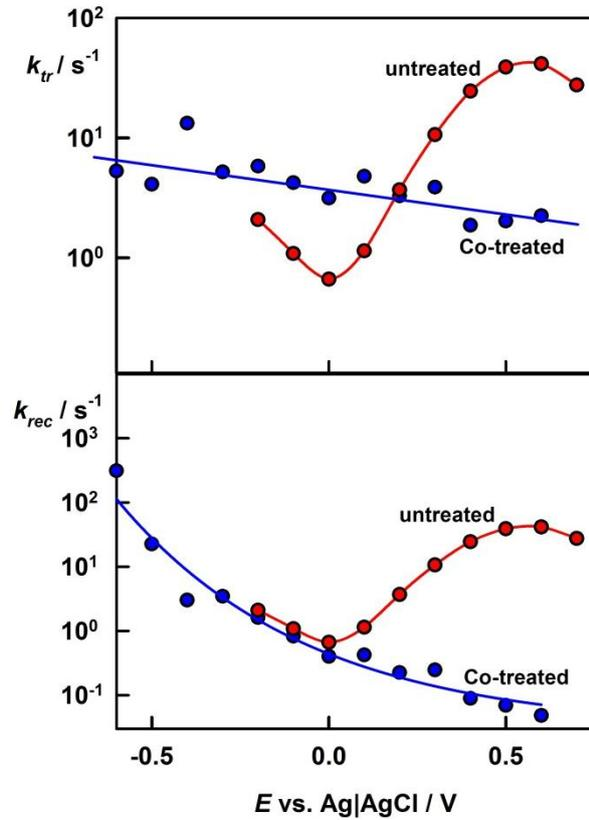
Figure 12. Rate constants for charge transfer and recombination for untreated and Co(II)-treated hematite film electrodes. Electrolyte 1.0 M NaOH. Illumination 455 nm, 11 mW cm<sup>-2</sup>. The treatment involved placing a drop of 10mM cobalt nitrate solution on the electrode surface for 60s, followed by rinsing with pure water for 30s.
