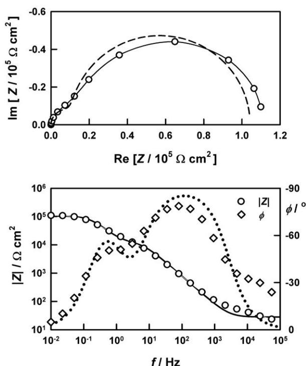
Figure 13. Typical experimental PEIS response for a thin film hematite photoanode. Electrolyte 1. NaOH. Potential 0.1 V vs. Ag|AgCl. Illumination 455 nm, ca.1 mW  $\text{cm}^{-2}$ .
