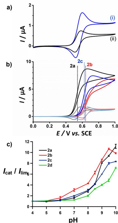
**Fig. 4** Cyclic voltammograms of : (a) 1 mM TEMPO without (i) and with (ii) cotton in ABS pH 4, potential scan rate 1  $\text{mVs}^{-1}$ ; (b) mediators 2a, 2b and 2c (1 mM) without and with cotton in CBS pH 10, scan rate 1  $\text{mVs}^{-1}$ . (c) Influence of pH on the efficiency of *N*-oxoammonium oxidation of cotton by electro-oxidized 2a (black), 2b (red), 2c (blue) and 2d (green).
