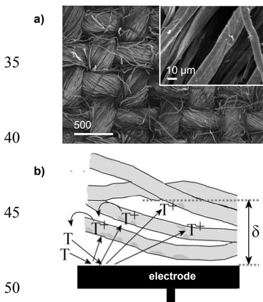
**Fig. 1** a) SEM images of cotton fabric, showing weave and fibre dimensions (inset) and (b) schematic drawing of mediator generation and reaction in the cotton fabric with diffusion layer thickness  $\delta$ .
