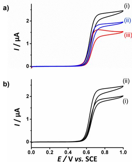
**Fig. 5** Cyclic voltammograms of cotton with 1 mM **2b** in (a) 0.1 M phosphate buffer pH 7 (i), 0.1 M citrate buffer (iii) and in phosphate/citrate mixed buffer pH 7 (ii); potential scan rate 1 mVs<sup>-1</sup>; (b) 0.2 M (i) and in 0.1 M phosphate buffer (ii), pH 7, potential scan rate 1 mVs<sup>-1</sup>.
