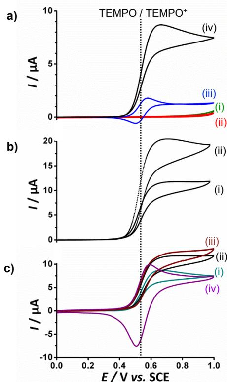
**Fig. 2** Cyclic voltammograms of (a) CBS (i), cotton with CBS (ii), 1 mM **2a** (iii) and cotton in CBS with 1 mM **2a** (iv) at pH 10; potential scan rate 1  $\text{mVs}^{-1}$ ; (b) cotton with 1 mM (i) and 2 mM **2a** (ii) in CBS pH 10, potential scan rate 10  $\text{mVs}^{-1}$ ; (c) cotton with 1 mM **2a** in CBS pH 10 at potential scan rates of (i) 1  $\text{mVs}^{-1}$ , (ii) 10  $\text{mVs}^{-1}$ , (iii) 20  $\text{mVs}^{-1}$ , and (iv) 100  $\text{mVs}^{-1}$ .
