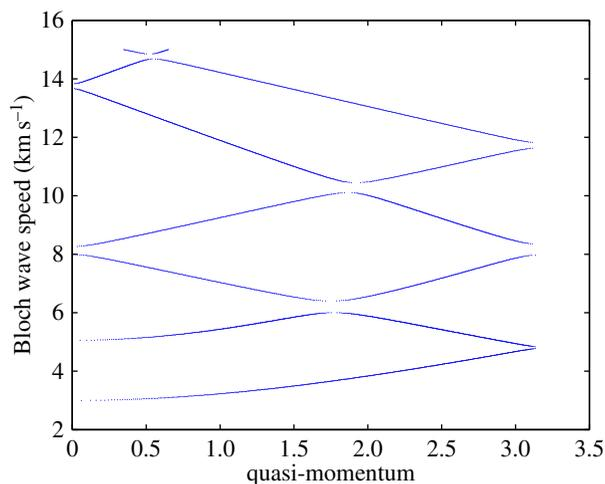
**Figure 3.** The dispersion relations (wave speed  $c = c(\theta)$  as a function of  $\theta \in [0, \pi)$ ) corresponding to the ‘in-plane’ part of the Bloch spectrum, see (4.2) Here the material parameters and  $h$  are the same as in figure 1,  $\hat{k} = 2.5$ . The values of  $c$  for  $\theta \in [\pi, 2\pi)$  are given by the formula  $c(\theta) = c(2\pi - \theta)$ . (Online version in colour.)
