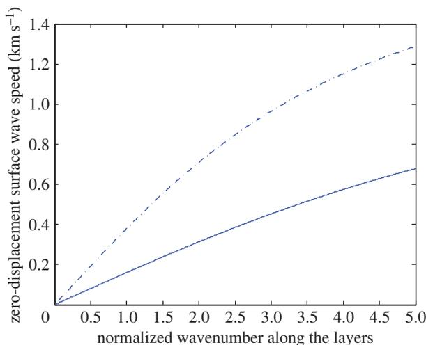
**Figure 2.** The Rayleigh-type wave speed  $c_{R,D}^h$  for the zero-displacement ('clamped') boundary, as a function of the parameter  $\hat{k}$ . For the solid line values of the material parameters are the same as in figure 1, for the dashed line the values of the material parameters are swapped between the materials A and B (equivalently, the order of the layers is BABAB. . . starting from the boundary). In both cases we set  $h = 0.1$ . (Online version in colour.)
