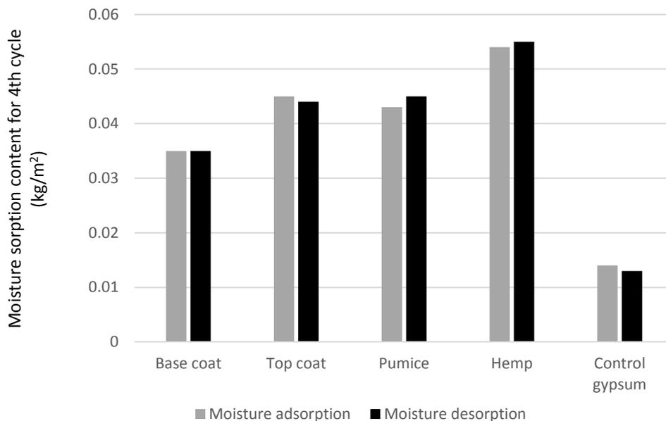
Figure 4. Moisture adsorption/desorption capacity of plaster specimens
