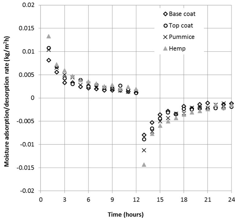
Figure 5. Moisture adsorption/desorption rate of clay coatings
