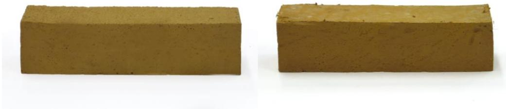
Figure 1. Base coat (left) and top coat (right) clay coating specimens
