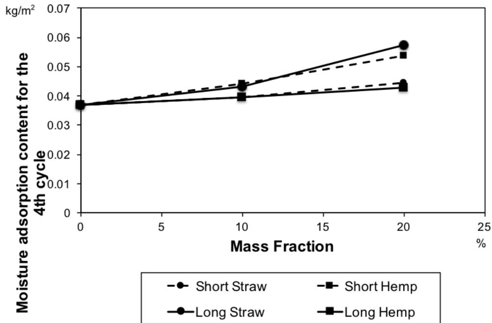
Figure 7 Moisture adsorption versus bio aggregate mass fraction
