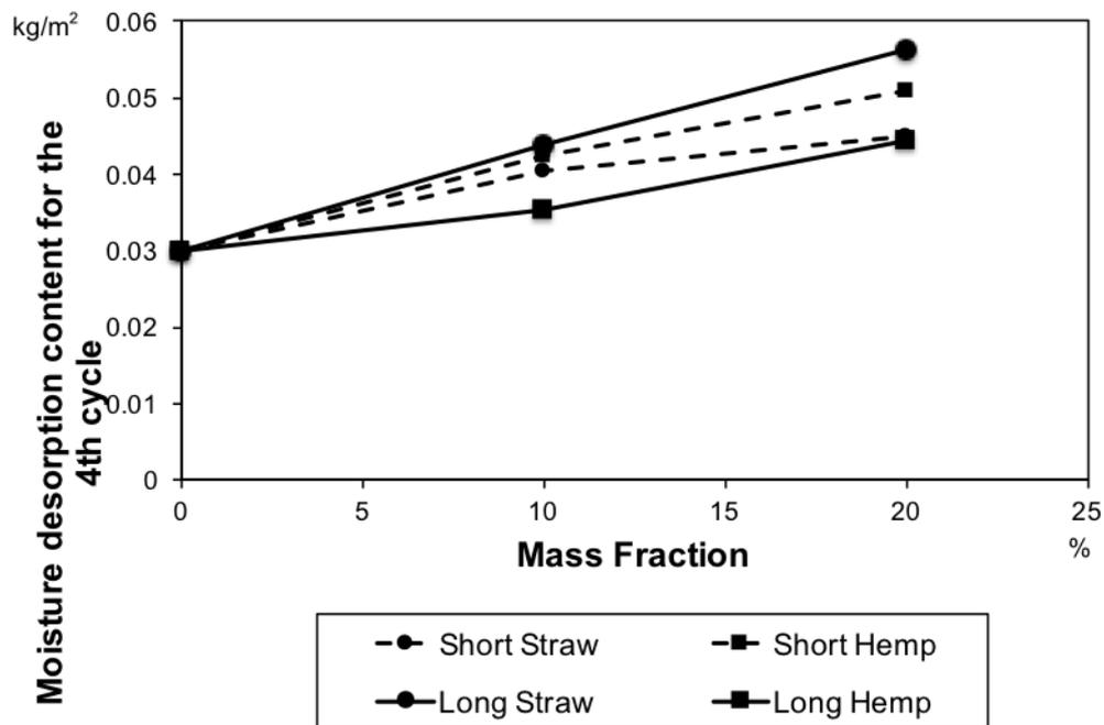
Figure 8 Moisture desorption versus bio aggregate mass fraction
