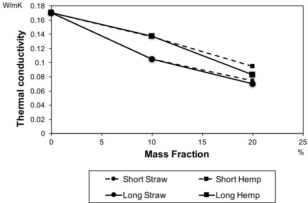
Figure 4 Thermal conductivity of lime-based coatings at 20°C
