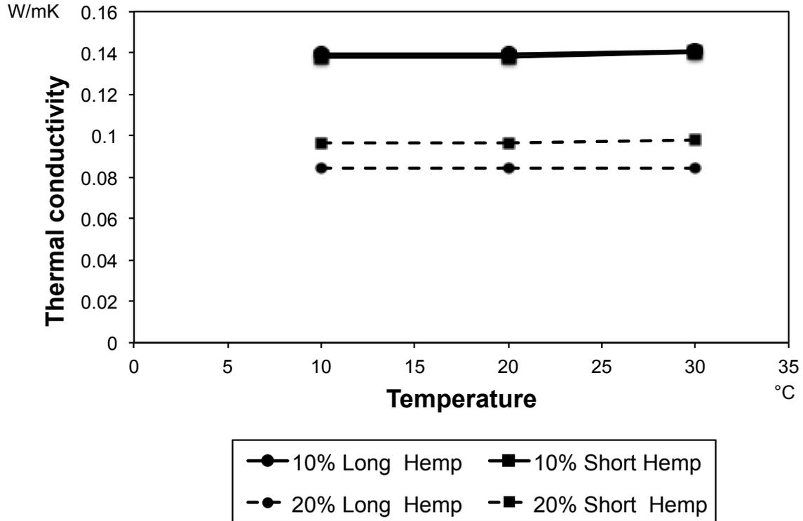
**Figure 6 Temperature dependent thermal conductivity of hemp and straw addition to lime-based coatings**
