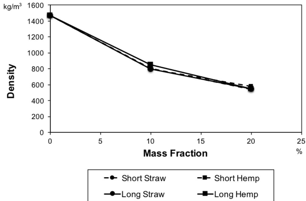
**Figure 1 Density versus bio aggregate mass fraction**
