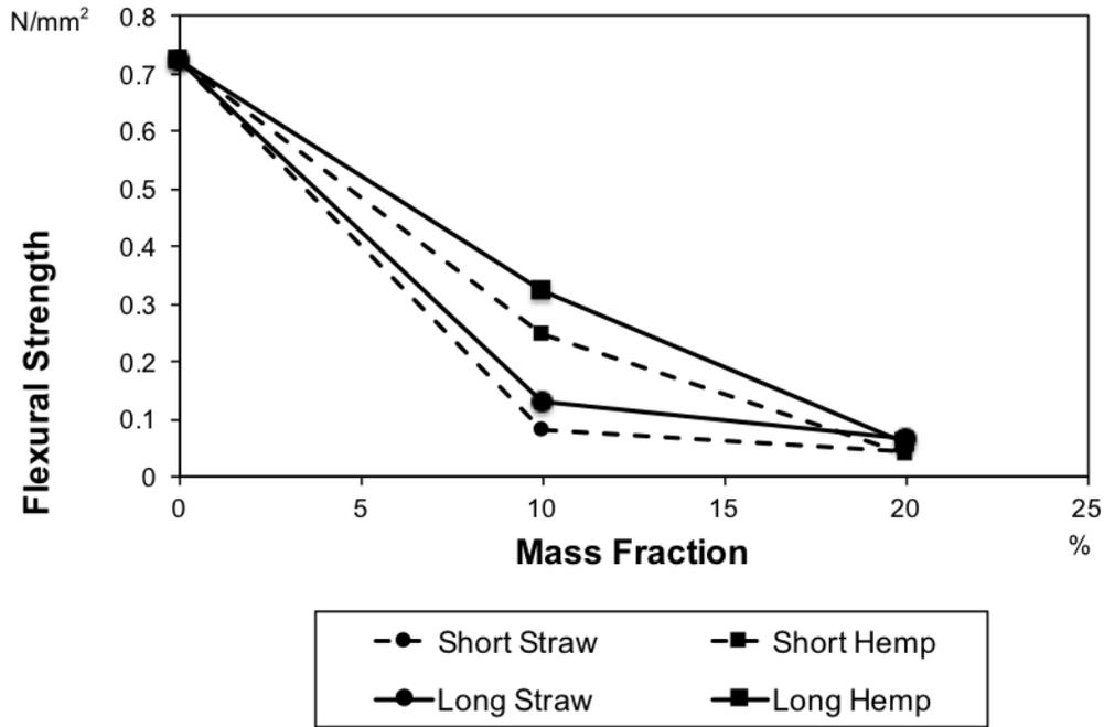
**Figure 2 Flexural strength versus bio aggregate mass fraction**
