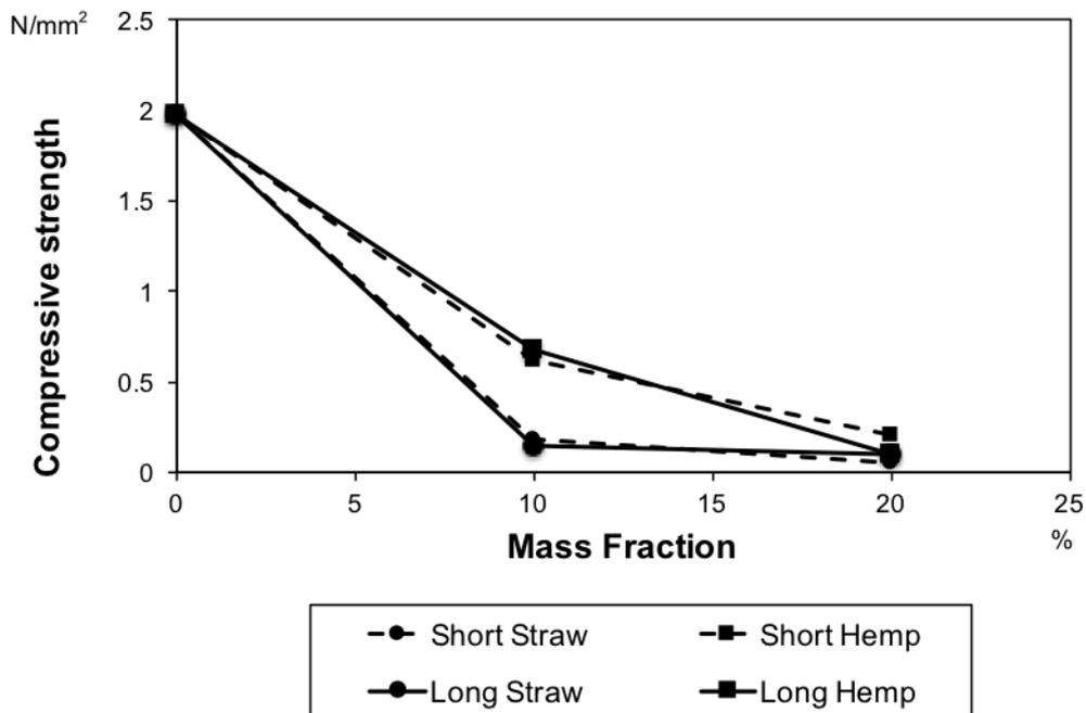
**Figure 3 Compressive strength versus bio aggregate mass fraction**
