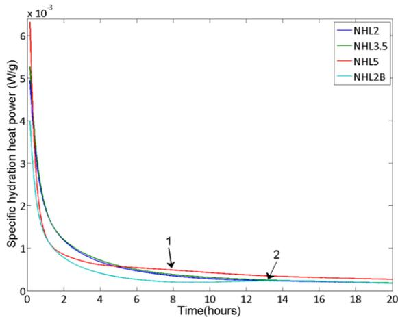
Figure 2. Calorimetric analysis for the first 20 hours.
