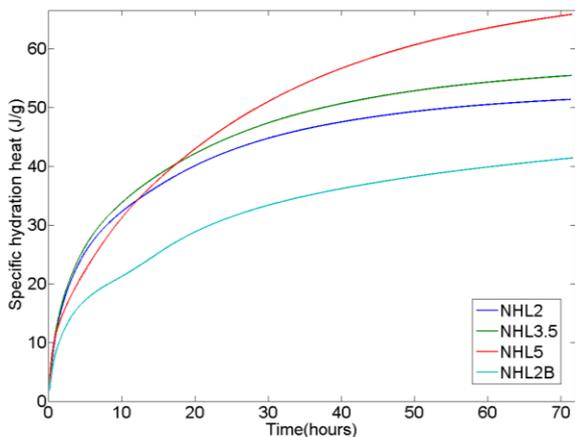
Figure 3. Specific hydration heat per 1 g of binder.
