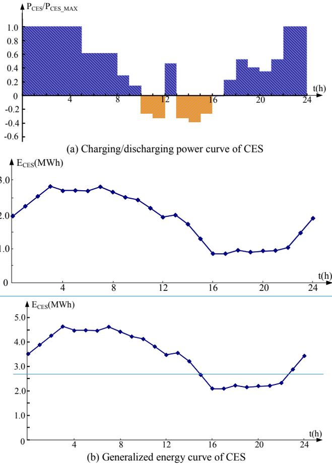
Fig. 7. Charging/discharging power and generalized energy of CES
