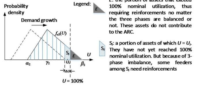
Fig. 3 The triangular distribution of feeders' nominal utilization rates after demand growth
