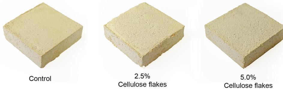
**Figure 1: Cement-lime Specimens**
