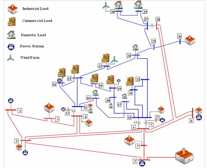
Fig 2. The IEEE 30 Bus Test System.
